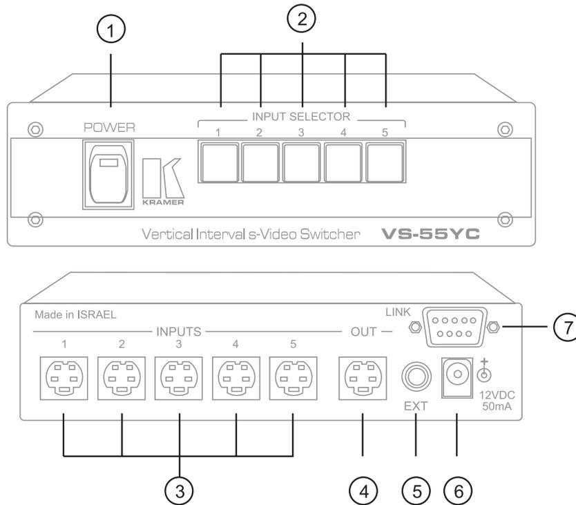
**Figure 4: VS-55YC Front and Rear Panel Features**
