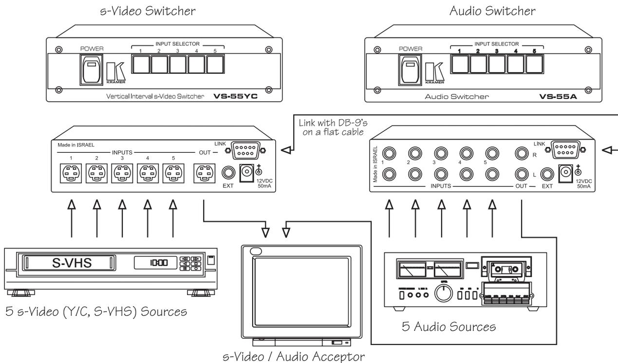
**Figure 6: Parallel Signal Switching**
