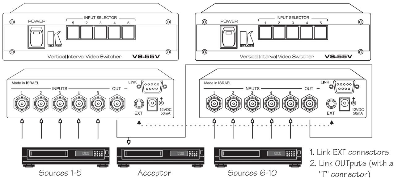
**Figure 5: Extending a Switcher – Adding inputs**
