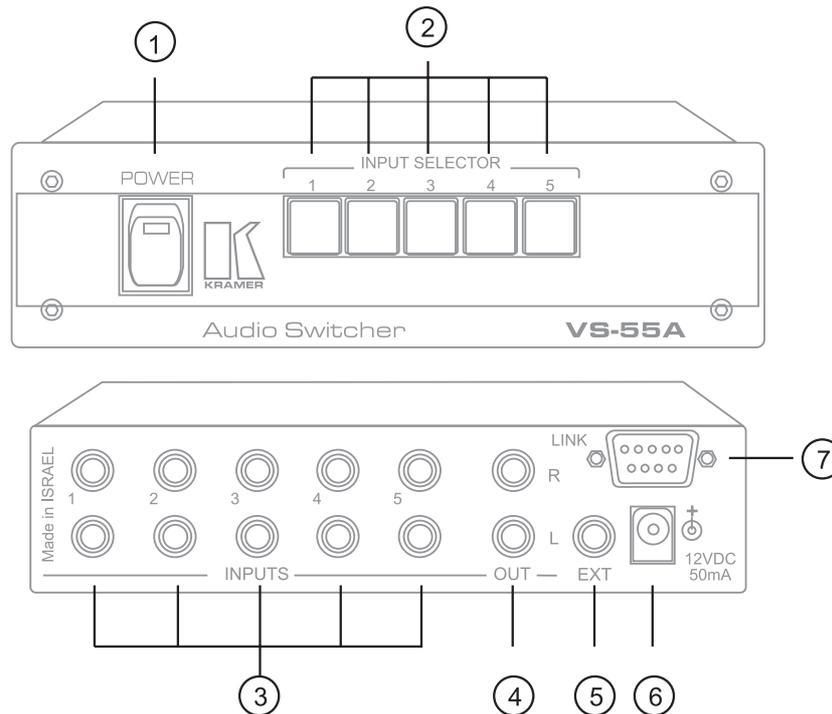
**Figure 2: VS-55A Front and Rear Panel Features**
